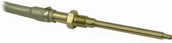
This sensor uses a K type Chromel/Alumel thermocouple and is intended for use in high temperature, high vibration environments. Control units and data loggers support K type thermocouples. The sensor is short and compact to minimise its susceptibility to vibration.
